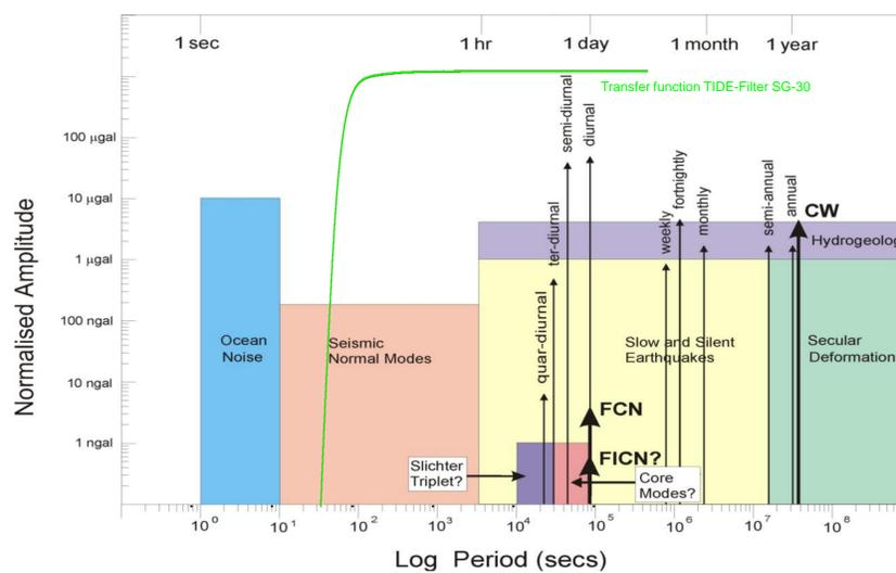
Spectral distribution of signals recorded with Superconducting gravimeters, after Crossley et. al., EOS, 1999. The green line indicates the frequency transfer function of an SG
