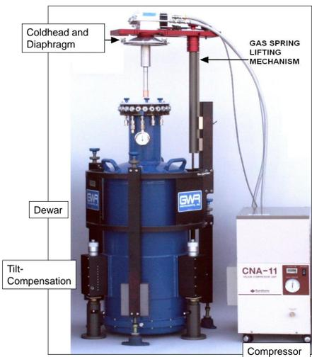
Present day observatory SG with a small dewar, efficient cooling system which allows to re-liquefy Helium gas. Cold head in lifted position. No transfer of liquid Helium is required during operation.
