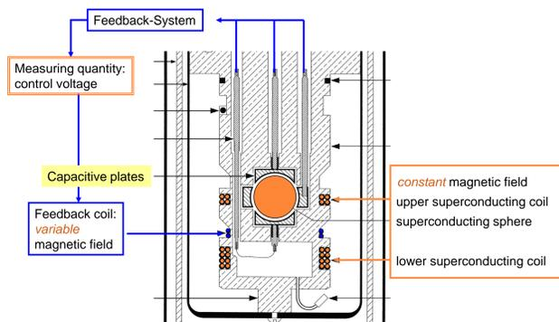
Cross section through the measuring system of a superconducting gravimeter
